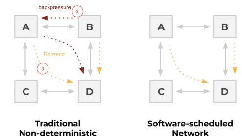
Figure 1: A traditional non-deterministic network compared to a Software-scheduled Network.
